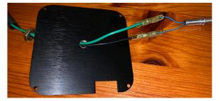
2. Once the wires are crimped to the probe, pass each butt splice (one at a time) through the mounting surface, washer and nut.
